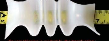
Severe thinning is evident by the translucency of the convolutions above. Permanently yieldi (stretching) PTFE beyond its elastic limit will compromise the materials mechanical integrity and can cause sudden premature failure.
